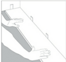
Step 1: Begin installation working from left to right. Insert 1/4" wide spacers at ends and edges where planks meet wall.
