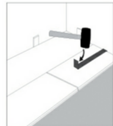
Step 8: Use hammer and pull bar to lock final piece in row. Insert spacer at end of row. Continue installation to final row.
