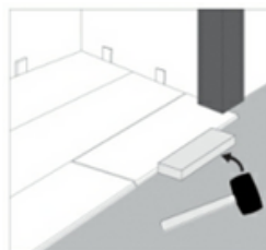
Step 1: Undercut door jamb to provide space to allow plank to slide freely. Tap long edge with hammer and tapping block to lock long edge.
